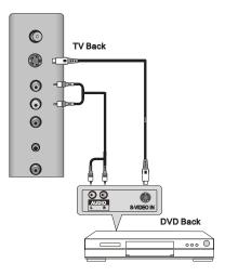
Connect the S-VIDEO output of the DVD or VCR to the S-VIDEO input on the set. The picture quality is improved; compared to connecting a regular VCR to the video input. Connect the Audio output of the DVD or VCR to the Audio input jacks on the set using the RCA cable.
